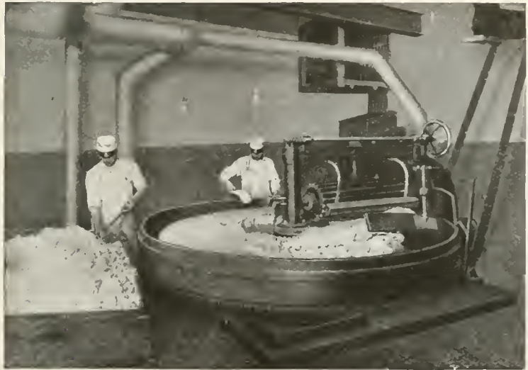
The mixture is chilled by contact with an ice water spray. After the whole mass has been permeated with the milk flavor it goes to the worker, where salt is added. When completely processed, it is packed in cartons or tubs. No hand touches the materials from start to finish.
